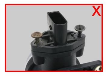
damage to cylinder housing, plug-in sensor, plug connection, strainer element, damage to screws.
