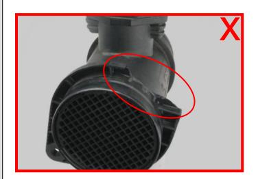
damage to cylinder housing, plug-in sensor, plug connection or strainer element  $\rightarrow$  not acceptable
